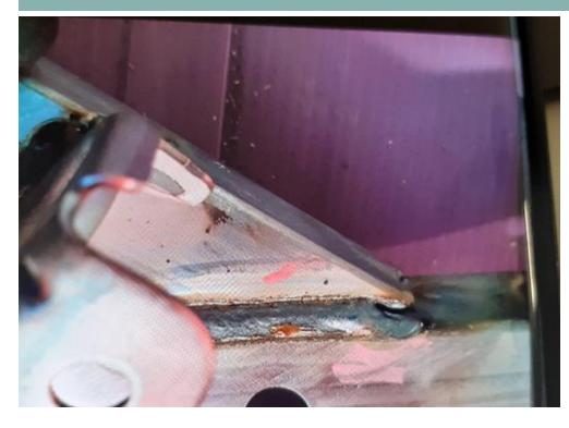
The picture shows a defect at the end of the welding seam.
